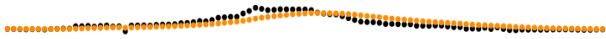
Fig. 12: Signal plot for x component of quaternion corresponding to upper left arm, in a sequence of body poses representing raising the left arm; black dots represent the raw signal taken from Kinect sensor while orange dots represent the filtered signal
